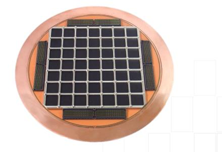
This SoW design posts significant challenges from defect inspection point of views from the algorithms and memory point of view comparing to other packaging.
