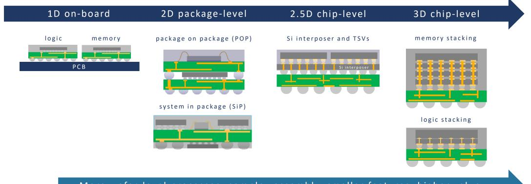
More wafer-level processes, complex assembly, smaller features, higher value
